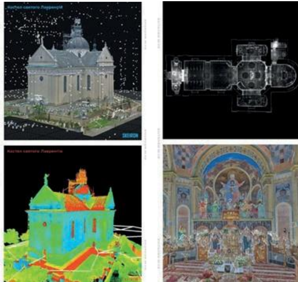
Fig. 1. Digitalization of cultural heritage objects in Ukraine: The Church of St. Lawrence in Zhovkva (1618) and the Church of St. Archangel Michael in Pidberizsi (1891-1910). Digitalizing: Lviv company "Skeiron", 2022. Source: Salstrom et al., 2024.
