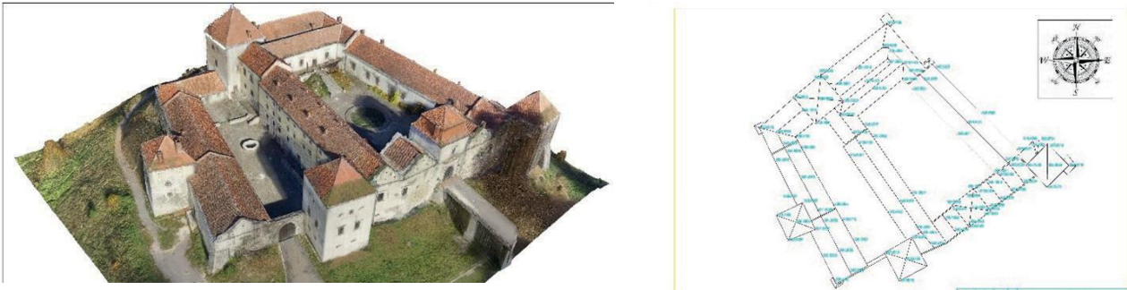
Fig. 3. Works on creating a detailed digital orthophoto plan of the roof of the Svirzh Castle. Scientific management Oliynyk O., Geodetic engineer D. V. Khomushko.
