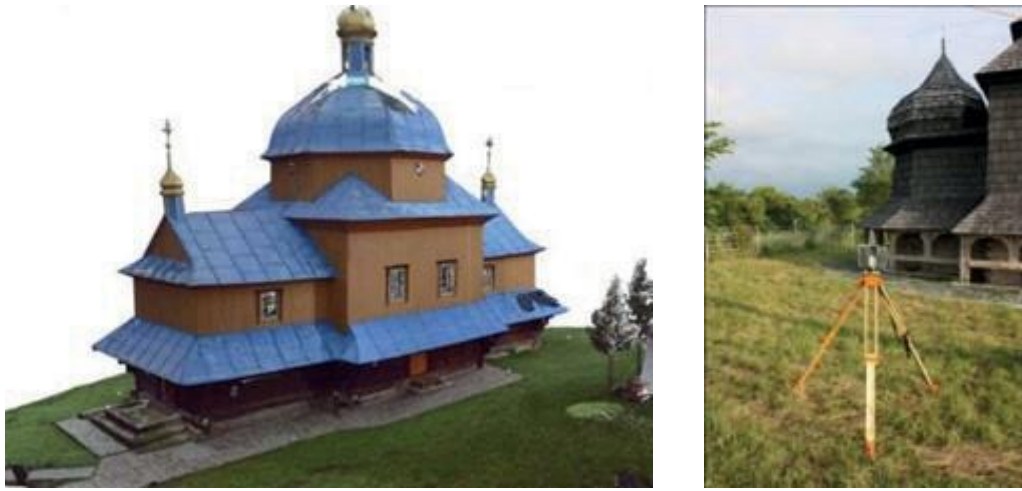
Fig. 7. Digital model of the wooden church Pr. Mother of God in the village Velikopole of Yavoriv district. Church scanning process. Source: https://geoterrace.lpnu.ua/
